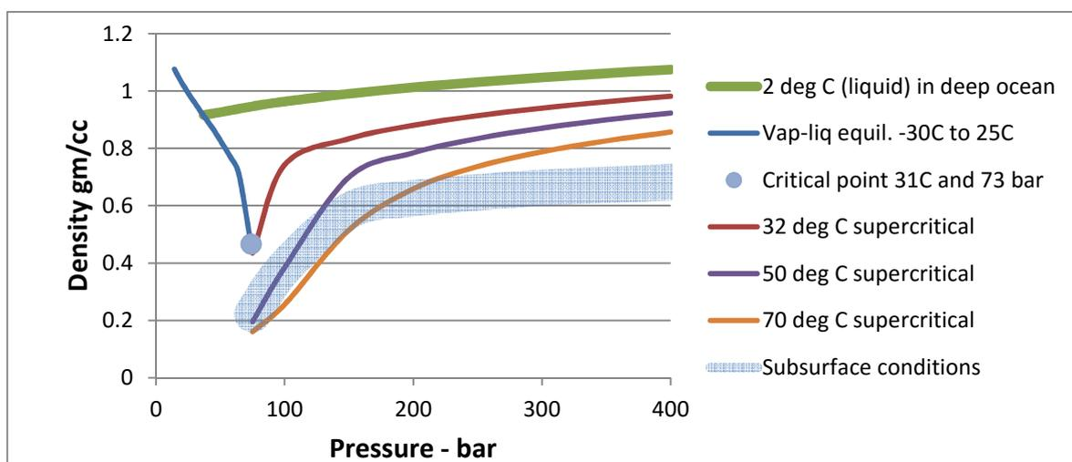
**Figure 6 Density vs. pressure for CO<sub>2</sub> at subcritical and supercritical temperatures**
