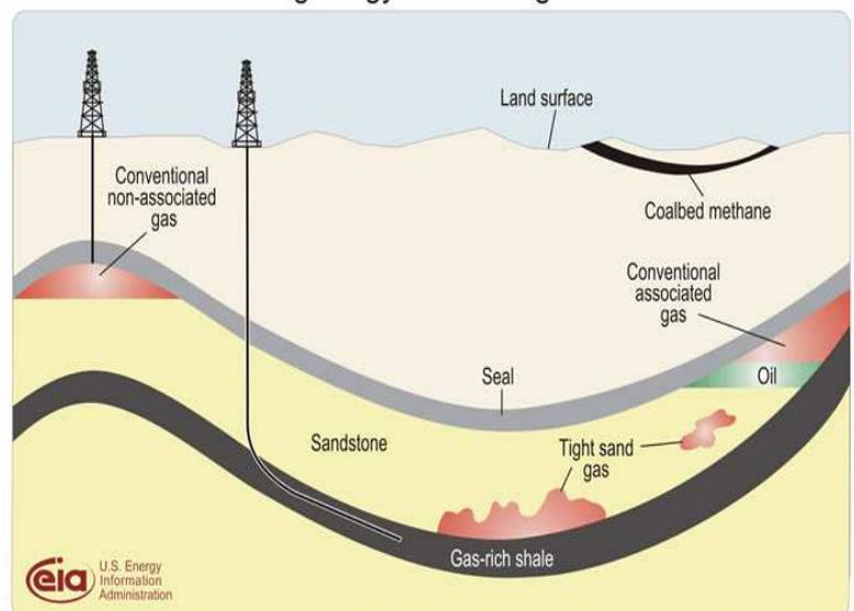
It is now economically viable and technically practicable to go beyond the natural accumulations of gas in capped porous rock near the surface and to drill deep into the hydrocarbon source rocks to access residual gas. Directional drilling now allows a gas well to follow the contours of gas-rich shale. Fracking<sup>1</sup> allows the gas to be liberated and drawn off at commercially viable rates. Also developments in LNG technology allow gas to be transported worldwide from inconvenient places.
